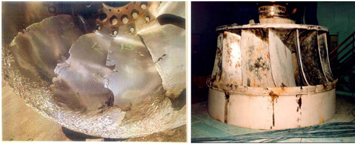
Fig. 1 Runner blades showing cavitation erosive failure (Ref 6)
